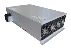
Bel Power Solutions offers a wide range of battery charger systems for railway applications consisting of adapted power supplies and appropriate temperature sensors. The batteries are charged according to the battery temperature and the properties of battery cells. When the battery is fully charged, it is maintained at the float charge voltage, which represents the optimum point for maximum available energy and optimum life expectancy of the battery.
