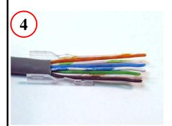
Lay wires into approx. positions in Load Bar
