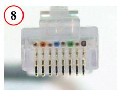
Ensure wires go all the way to front of housing
