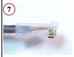
Insert wires and Load Bar into housing
