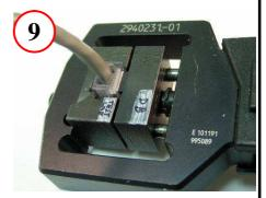
Crimp wires and strain relief
