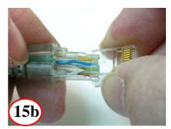
Place load bar assembly into housing
