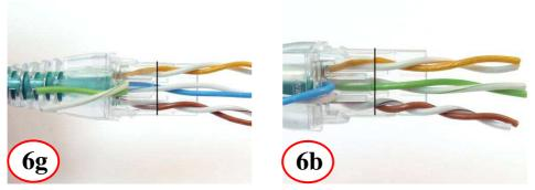
Check wire alignment – here, Org is aligned wrong, needs ½ twist
