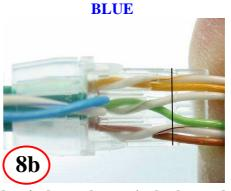
Untwist lower three pairs back to ends of side walls. Spread Grn pair
