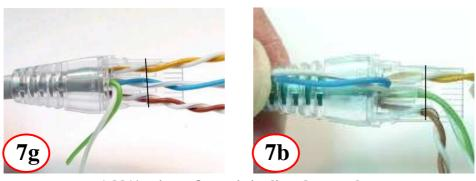
Add ½ twist so Org pair is aligned correctly – PAIRS MUST HAVE ½ to 1 TWIST ONLY
