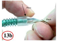
Pinch load bar end, then press on back to set wires in place
