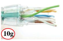
Check Grn pair for alignment Add 1/2 twist if necessary
