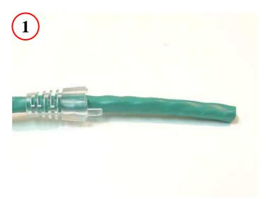
Slide Strain Relief onto cable
