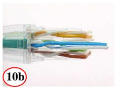
Check Blu pair for alignment Add 1/2 twist if necessary
