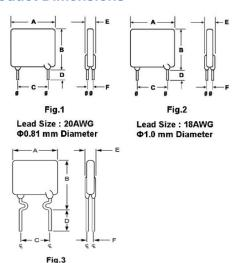
Lead Size : 20AWG Ф0.81 mm Diameter
