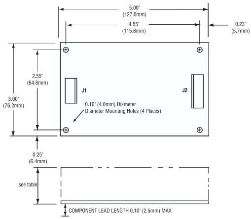
Figure 5. Mechanical Drawing
