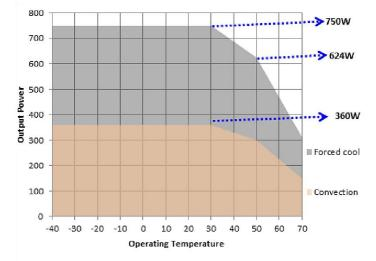
Forced air cooled load: 750 W up to  $30^{\circ}$ C De-rate between  $30-50^{\circ}$ C @ 0.8375% per °C De-rate above  $50^{\circ}$ C @ 2.5% per °C
