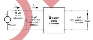
Figure 21. Test setup for measuring input reflected ripple currents, ic and is.
