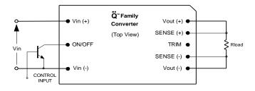
Figure 1. Circuit configuration for ON/OFF function.
