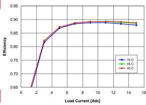
Figure 15. Efficiency vs. load current and ambient temperature for convert-er mounted horizontally with Vin = 27 V and air flowing from pin 3 to pin 4 at a rate of 200 LFM (1.0 m/s).
