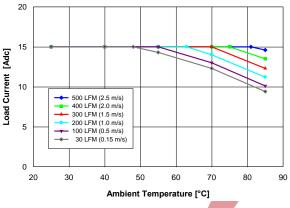
20 15 Load Current [Adc] 10 500 LFM (2.5 m/s) 400 LFM (2.0 m/s) 300 LFM (1.5 m/s) 200 LFM (1.0 m/s) 100 LFM (0.5 m/s) 30 LFM (0.15 m/s) 0 20 30 40 50 60 70 80 90 Ambient Temperature [°C]
