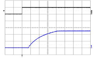
Figure 17. Turn-on transient at full rated load current (resistive) plus 10,000 F at Vin = 24 V, triggered via ON/OFF pin. Top trace: ON/OFF signal (5 V/div.). Bottom trace: output voltage (2 V/div.). Time scale: 2 ms/div.
