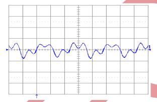
Figure 20. Output voltage ripple (20 mV/div.) at full rated load current into a resistive load with Co = 10 μF tantalum + 1μF ceramic and Vin = 24 V. Time scale: 1 μs//div.
