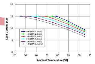
Figure 10. Available load current vs. ambient temperature and airflow rates for converter mounted horizontally with Vin = 27 V, air flowing from pin 3 to pin 4 and maximum FET temperature ≤ 120 °C.
