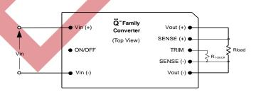
Figure 4. Configuration for decreasing output voltage.
