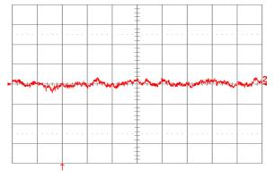
Figure 23. Input reflected ripple current, is (10 mA/div), measured through 10 µH at the source at full rated load current and Vin = 24 V. Re-fer to Fig. 23 for test setup. Time scale: 1 µs/div.
