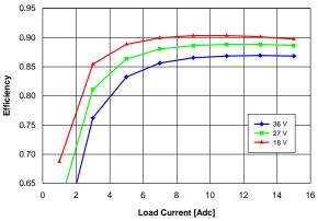
Figure 12. Efficiency vs. load current and input voltage for converter mounted vertically with air flowing from pin 3 to pin 1 at a rate of 300 LFM (1.5 m/s) and Ta = 25 °C
