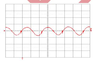
Figure 22. Input reflected ripple current, ic (100 mA/div), measured at input terminals at full rated load current and Vin = 24 V. Refer to Fig. 21 for test setup. Time scale: 1 µs /div.
