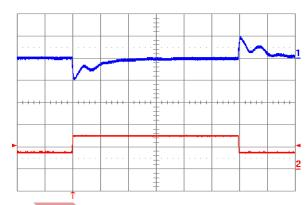
Figure 19. Output voltage response to load current stepchange (3.75 A – 7.5 A – 3.75 A) at Vin = 24 V. Top trace: output voltage (100 mV/div.). Bottom trace: load current (5 A/div). Current slew rate: 5 A/ μs . Co = 450 μF tantalum + 1 μF ceramic. Time scale: 0.2 m
