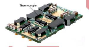
Figure 26. Location of the thermocouple for thermal testing.
