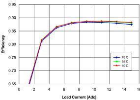
Figure 13. Efficiency vs. load current and ambient temperature for convert-er mounted vertically with Vin = 27 V and air flowing from pin 3 to pin 1 at a rate of 200 LFM (1.0 m/s).
