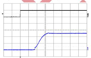
Figure 16. Turn-on transient at full rated load current (resistive) with no out-put capacitor at Vin = 24 V, triggered via ON/OFF pin. Top trace: ON/OFF signal (5 V/div.). Bottom trace: output voltage (2 V/div.) Time scale: 1 ms/div.
