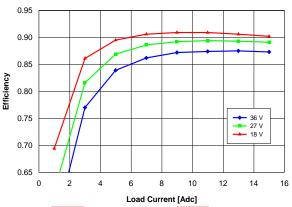
Figure 14. Efficiency vs. load current and input voltage for converter mounted horizontally with air flowing from pin 3 to pin 4 at a rate of 300 LFM (1.5 m/s) and Ta = 25 °C.
