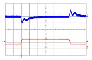
Figure 18. Output voltage response to load current stepchange (3.75 A – 7.5 A – 3.75 A) at Vin = 24 V. Top trace: output voltage (100 mV/div). Bottom trace: load current (5 A/div.). Current slew rate: 0.1 A/ μs . Co = 1 μF ceramic. Time scale: 0.2 ms/div.
