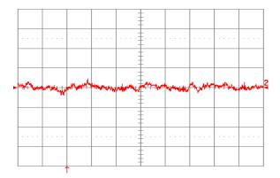
Figure 23. Input reflected ripple current, is (10 mA/div), measured through 10 µH at the source at full rated load current and Vin = 24 V. Re-fer to Fig. 21 for test setup. Time scale: 1 µs/div.
