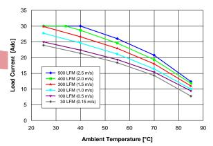
Figure 11. Available load current vs. ambient temperature and airflow rates for converter mounted horizontally with Vin = 27 V, air flowing from pin 3 to pin 4 and maximum FET temperature ≤ 105 °C.
