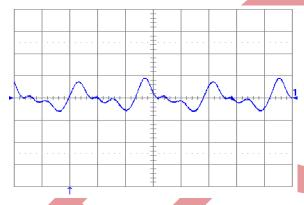
Figure 20. Output voltage ripple (20 mV/div.) at full rated load current into a resistive load with Co = 10 μF tantalum + 1μF ceramic and Vin = 24 V. Time scale: 1 μs/div.
