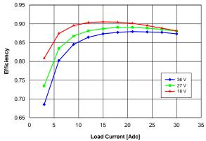
Figure 12. Efficiency vs. load current and input voltage for converter mounted vertically with air flowing from pin 3 to pin 1 at a rate of 300 LFM (1.5 m/s) and Ta = 25 °C
