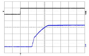
Figure 17. Turn-on transient at full rated load current (resistive) plus 10,000 µF F at Vin = 24 V, triggered via ON/OFF pin. Top trace: ON/OFF signal (5 V/div.). Bottom trace: output voltage (1 V/div.). Time scale: 1 ms/div.
