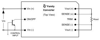
Figure 1. Circuit configuration for ON/OFF function.
