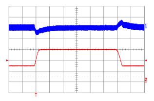
Figure 18. Output voltage response to load current stepchange (7.5 A – 15 A – 7.5 A) at Vin = 24 V. Top trace: output voltage (100 mV/div). Bottom trace: load current (5 A/div.). Current slew rate: 0.1 A/ μs. Co = 1 μF ceramic. Time scale: 0.2 ms/div..
