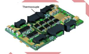
Figure 26. Location of the thermocouple for thermal testing.
