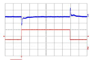
Figure 19. Output voltage response to load current stepchange (7.5 A – 15 A – 7.5 A) at Vin = 24 V. Top trace: output voltage (100 mV/div.). Bottom trace: load current (5 A/div). Current slew rate: 5 A/ μs. Co = 450 μF tantalum + 1 μF ceramic. Time scale: 0.2 ms/d
