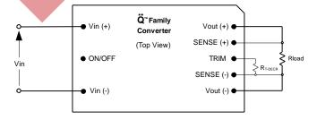
Figure 4. Configuration for decreasing output voltage.
