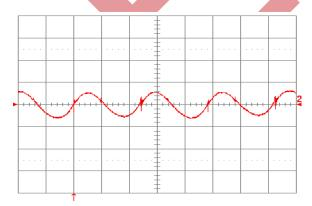
Figure 22. Input reflected ripple current, ic (100 mA/div), measured at input terminals at full rated load current and Vin = 24 V. Refer to Fig. 21 for test setup. Time scale: 1 µs/div.
