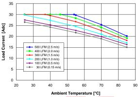
Figure 10. Available load current vs. ambient temperature and airflow rates for converter mounted horizontally with Vin = 27 V, air flowing from pin 3 to pin 4 and maximum FET temperature ≤ 120 °C.
