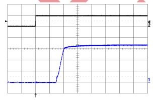
Figure 16. Turn-on transient at full rated load current (resistive) with no out-put capacitor at Vin = 24 V, triggered via ON/OFF pin. Top trace: ON/OFF signal (5 V/div.). Bottom trace: output voltage (1 V/div.) Time scale: 1 ms/div.
