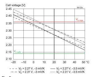
Float charge voltage vs temp. for different temp. coefficients.
