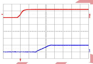
Fig. 0.7525V.4: Turn-on transient for Vout = 0.7525 V with application of Vin at full rated load current (resistive) and 100 μF external capacitance at Vin = 12 V. Top trace: Vin (10 V/div.); Bottom trace: output voltage (1 V/div.); Time scale: 2 ms/div.
