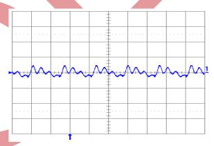
Fig. 1.5V.5: Output voltage ripple (20 mV/div.) at full rated load current into a resistive load with external capacitance  $100 \,\mu$ F ceramic + 1  $\mu$ F ceramic and Vin = 12 V for Vout = 1.5 V. Time scale: 2  $\mu$ s/div.
