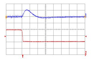
Fig. 0.7525V.7: Output voltage response for Vout = 0.7525 V to negative load current step change from 20 A to 10 A with slew rate of -5 A/μs at Vin = 12 V. Top trace: output voltage (200 mV/div.); Bottom trace: load current (5 A/div.). Co = 100 μF ceramic. Time scale: 20 μs/div.
