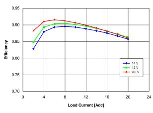
Fig. 1.8V.2: Efficiency vs. load current and input voltage for Vout = 1.8 V converter mounted vertically with air flowing at a rate of 200 LFM (1 m/s) and Ta = 25 °C.
