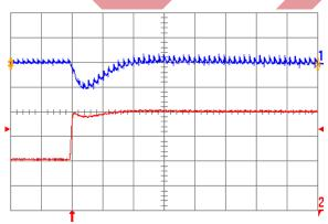
Fig. 1.5V.6: Output voltage response for Vout = 1.5 V to positive load current step change from 10 A to 20 A with slew rate of 5 A/ $\mu$ s at Vin = 12 V. Top trace: output voltage (200 mV/div.); Bottom trace: load current (5 A/div.). Co = 100  $\mu$ F ceramic. Time scale: 20  $\mu$ s/div.
