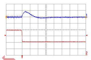
Fig. 1.2V.7: Output voltage response for Vout = 1.2 V to negative load current step change from 20 A to 108 A with slew rate of -5 A/ $\mu$ s at Vin = 12 V. Top trace: output voltage (200 mV/div.); Bottom trace: load current (5 A/div.). Co = 100  $\mu$ F ceramic. Time scale: 20  $\mu$ s/div.
