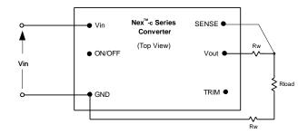
Fig. B: Remote sense circuit configuration.
