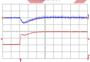
Fig. 0.7525V.6: Output voltage response for Vout = 0.7525 V to positive load current step change from
