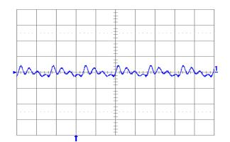
Fig. 1.2V.5: Output voltage ripple (20 mV/div.) at full rated load current into a resistive load with external capacitance 100 μF ceramic + 1 μF ceramic and Vin = 12 V for Vout = 1.2 V. Time scale: 2 μs/div.
