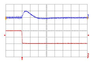
Fig. 1.5V.7: Output voltage response for Vout = 1.5 V to negative load current step change from 20 A to 10 A with slew rate of -5 A/μs at Vin = 12 V. Top trace: output voltage (200 mV/div.); Bottom trace: load current (5 A/div.). Co = 100 μF ceramic. Time scale: 20 μs/div.
