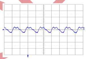
Fig. 2.5V.5: Output voltage ripple (20 mV/div.) at full rated load current into a resistive load with external capacitance  $100 \,\mu\text{F}$  ceramic + 1  $\mu\text{F}$  ceramic and Vin = 12 V for Vout = 2.5 V. Time scale: 2  $\mu$ s/div.
