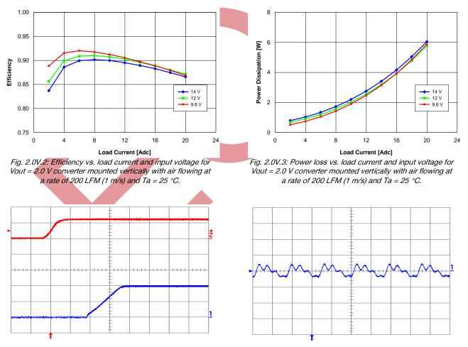
Fig. 2.0V.4: Turn-on transient for Vout = 2.0 V with application of Vin at full rated load current (resistive) and 100  $\mu$ F external capacitance at Vin = 12 V. Top trace: Vin (10 V/div.); Bottom trace: output voltage (1 V/div.); Time scale: 2 ms/div.
