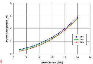
Fig. 1.5V.3: Power loss vs. load current and input voltage for Vout = 1.5V converter mounted vertically with air flowing at a rate of 200 LFM (1 m/s) and Ta = 25 °C.
