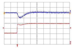
Fig. 1.2V.6: Output voltage response for Vout = 1.2 V to positive load current step change from 10 A to 20 A with slew rate of 5 A/ $\mu$ s at Vin = 12 V. Top trace: output voltage (200 mV/div.); Bottom trace: load current (5 A/div.). Co = 100  $\mu$ F ceramic. Time scale: 20  $\mu$ s/div.
