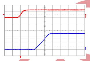
Fig. 2.5V.4: Turn-on transient for Vout = 2.5 V with application of Vin at full rated load current (resistive) and 100 μF external capacitance at Vin = 12V. Top trace: Vin (10 V/div.); Bottom trace: output voltage (1 V/div.); Time scale: 2 ms/div.
