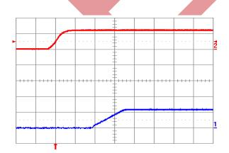
Fig. 1.2V.4: Turn-on transient for Vout = 1.2 V with application of Vin at full rated load current (resistive) and 100 μF external capacitance at Vin = 12 V. Top trace: Vin (10 V/div.); Bottom trace: output voltage (1 V/div.); Time scale: 2 ms/div.
