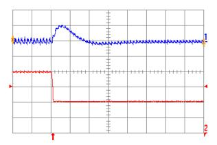
Fig. 2.5V.7: Output voltage response for Vout = 2.5 V to negative load current step change from 20 A to 10 A with slew rate of -5A/μs at Vin = 12 V. Top trace: output voltage (200 mV/div.); Bottom trace: load current (5 A/div.). Co = 100 μF ceramic. Time scale: 20 μs/div.
