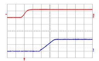
Fig. 1.8V.4: Turn-on transient for Vout = 1.8 V with application of Vin at full rated load current (resistive) and 100 μF external capacitance at Vin = 12 V. Top trace: Vin (10 V/div.); Bottom trace: output voltage (1 V/div.); Time scale: 2 ms/div.
