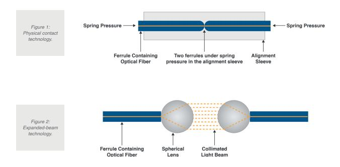
Expanded-beam fiber optic connectors utilize a lens to expand and collimate the light emitting from an optical fiber. This collimated light beam is transmitted through an air gap to a mating connector, where the light is collected and focussed by a second lens into a second optical fiber to complete the connection. Improving Communication Connectivity Within Explosive Atmosphere Applications
